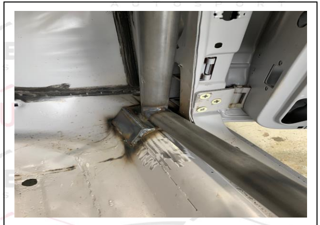
PHOTO 6 FRONT ROLLBAR TO FLOOR ATTACHMENT
