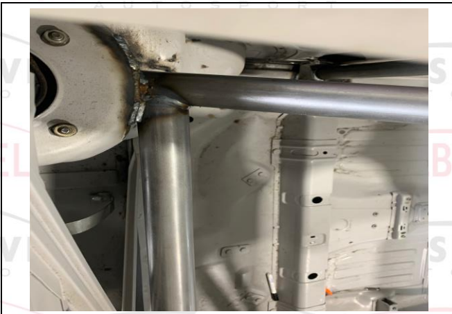
PHOTO 5 REAR BACKSTAY TO BODYSHELL ATTACHMENT
