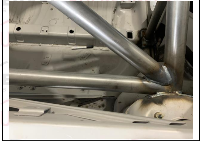
PHOTO 13 SHOULDER HARNESS ATTACHMENT - CO DRIVER
