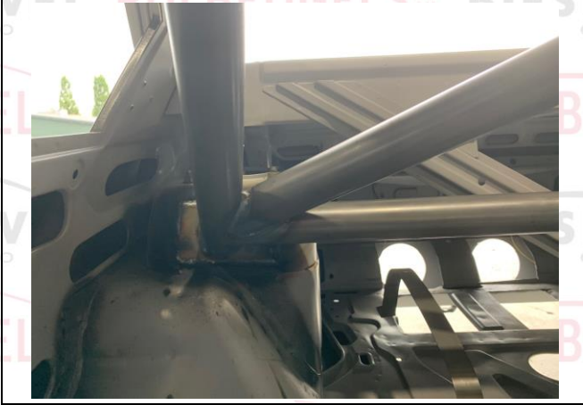
PHOTO 12 SHOULDER HARNESS ATTACHMENT - DRIVER
