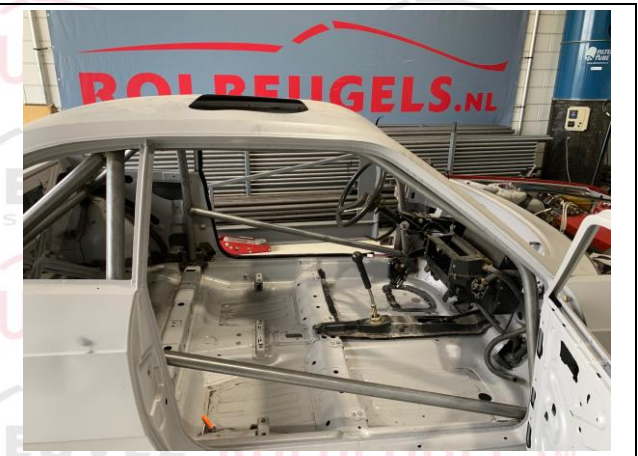
PHOTO 11 ANTI-INTRUSION DOORBAR – CO-DRIVER
