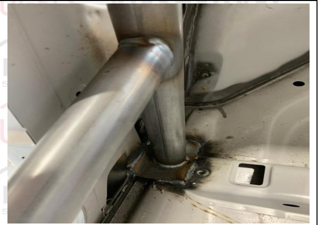
PHOTO 4 MAIN ROLLBAR TO FLOOR ATTACHMENT
